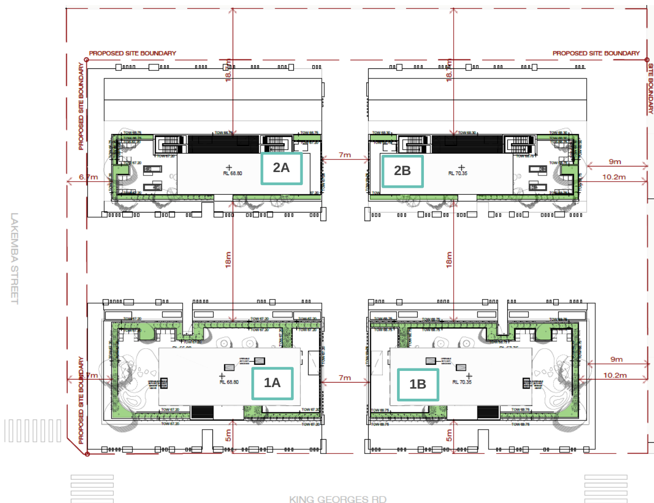
Figure 3 – Roof Plan with buildings numbered
